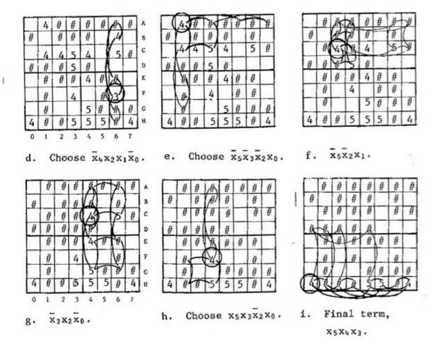
Figure 8-5 The Weight Algorithm for a Six-Variable Function
